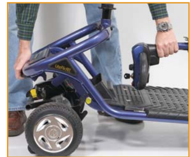
While squeezing the release lever, pull up on the rear frame
